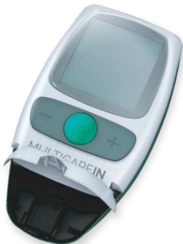
For glucose measurement it is not necessary a particular cleaning procedure, only if blood or other material (debris, dust, etc..) come into direct contact with the plastic support of the device. If so, wipe the device surface with a soft cloth dampened with 70% alcohol solution.
