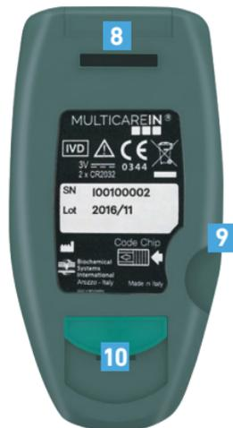
8. Battery housing: sliding cover for batteries replacement.
